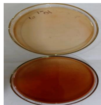
Photo 15: Fiehe's test- cherry-red positive (lower petri dish)
